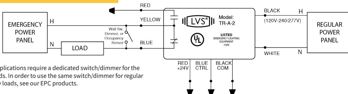
Note: Shunt applications require a dedicated switch/dimmer for the emergency loads. In order to use the same switch/dimmer for regular and emergency loads, see our EPC products.
