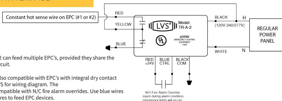
Note: One TR-A-2 can feed multiple EPC's, provided they share the same sensing circuit.
