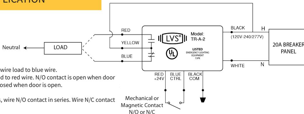
Note 1: For N/O contact, wire load to blue wire. For N/C contact, wire load to red wire. N/O contact is open when door is open. N/C contact is closed when door is open.
