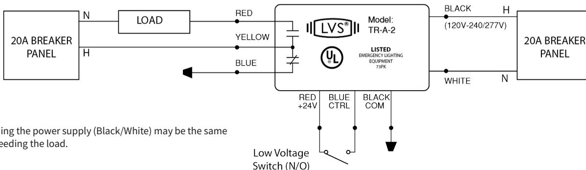
Note: Panel feeding the power supply (Black/White) may be the same from the panel feeding the load.
