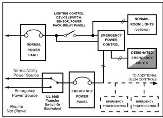
**Wiring Diagram:** A common dimmer controls both normal and emergency lighting in a space. Upon loss of normal power, the emergency lighting comes on at full brightness regardless of dimmer position.
