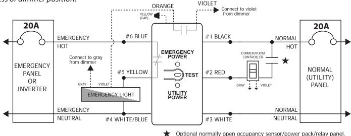
**Wiring Diagram #2 (Shunt):** A dedicated dimmer (fed by emergency power) controls emergency lighting in a space. Upon loss of normal power, the emergency lighting comes on at full brightness regard-less of dimmer position.
