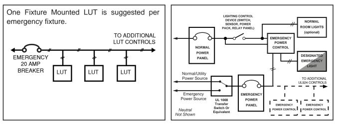
**Wiring Diagram #1 (Suggested):** A dimmer (fed by normal power) controls emergency lighting in a space. Upon loss of normal power, the emergency lighting comes on at full brightness regard-less of dimmer position.
