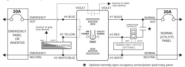
**Wiring Diagram #2 (Shunt):** A dedicated dimmer controls emergency lighting in a space. Upon loss of normal power, the emergency lighting comes on at full brightness regardless of dimmer position.
