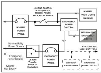
**Wiring Diagram #1 (Suggested):** A common dimmer controls both normal and emergency lighting in a space. Upon loss of normal power, the emergency lighting comes on at full brightness regardless of dimmer position.
