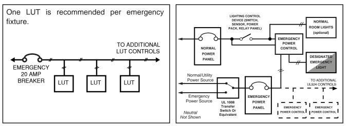
**Wiring Diagram #1 (Suggested):** A common switch controls both normal and emergency lighting in a space. Upon loss of normal power, the emergency lighting comes on regardless of switch position.
