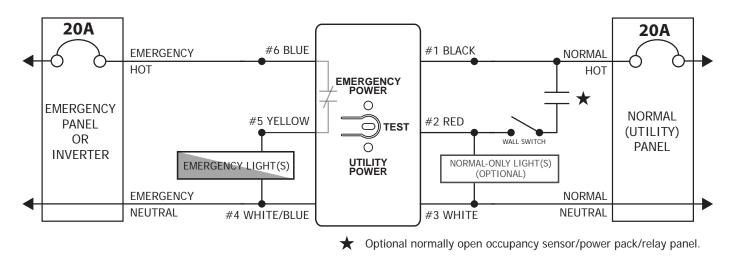
**Wiring Diagram #2 (Shunt):** A dedicated switch controls emergency lighting in a space. Upon loss of normal power, the emergency lighting comes on regardless of switch position.
