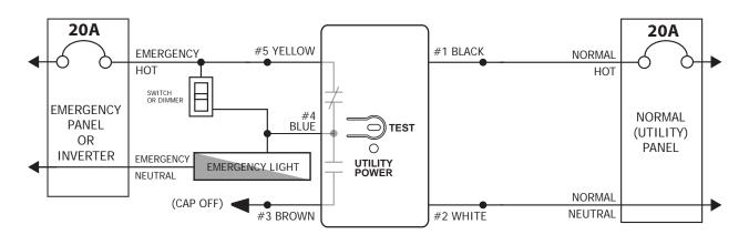
**Wiring Diagram #2:** For use with Lutron Vive integral fixture controls and DALI drivers with self powered DALI link, such as Philips® SR XI040C110V054VPT1 and XI075C200V054VPT1 and Osram ® Dexal (tm) OTi50/120-277/1A4 DX L and OTi30/120-277/1A0 DX L
