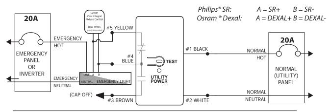
**Wiring Diagram #3:** For use with Lutron Vive integral fixture controls and EcoSystem drivers without self powered DALI link, such as Lutron LDE1, LDE5, L3D, and L3D0
