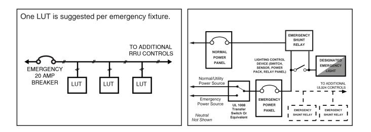
**Wiring Diagram #1:** A dedicated switch or line voltage dimmer controls emergency lighting in a space. Upon loss of normal power, the emergency lighting comes on at full brightness regardless of switch or dimmer position. NOTE: LUT-SHUNT-FM is not for use with 0-10V DIMMER. Use LUT-SHUNT-D-FM.
