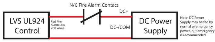
LVS products with Fire Alarm Tie-In ship with a low voltage wire red loop. Red loop can be cut and connected as shown below. Red wires are polarity independent.
