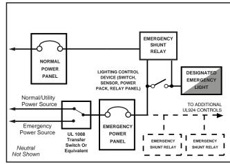
**Wiring Diagram #1:** A dedicated switch or line voltage dimmer controls emergency lighting in a space. Upon loss of normal power, the emergency lighting comes on at full brightness regardless of switch or dimmer position. NOTE: RRU-UNV-FM is not for use with 0-10V DIMMER. Use RRU-X-UNV-FM.
