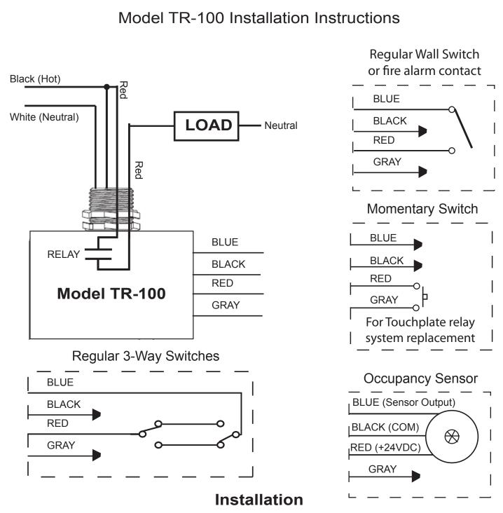
In order to install the TR-100 in accordance with national/local code requirements, a qualified electrician should review and understand the installation instructions: Check voltage and current requirements. Review wiring diagram and connect wires, one group at a time, in accordance with the numeric identification.
